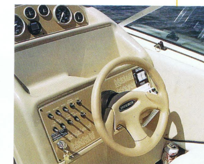
The helm station offers great visibility, full instrumentation. Compass, trim tabs and digital depth sounder are standard.
